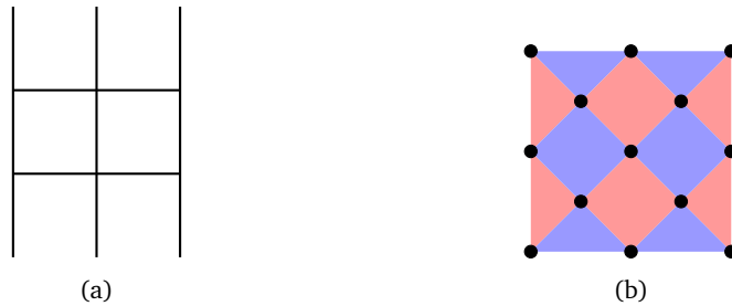
Figure 6.2: Graphical depiction of the original surface code. In (a), qubits are located on edges. Z -type stabilizers involve all qubits around a plaquette, including the open plaquettes at the top and bottom. Called “rough boundaries”, these are weight-three stabilizers. X -type stabilizers involve all qubits around a vertex. The weight three X -type stabilizers on the left and right form the “smooth” boundaries. The logical X operator can be taken to be the X operator acting on all three qubits on the top, while the logical Z operator can be taken to be the Z operator acting on all three qubits on the left. Panel (b) shows the same stabilizers in our previous format. The rotation of the two versions of the surface code relative to each other is immediately apparent.
