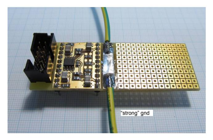
Figure 8 Example: gnd over wires.
