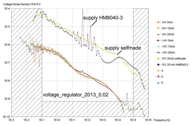
Figure 1 Voltage Noise Density of one prototype and two other supplies
