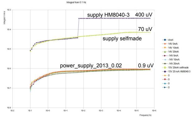
Figure 2 Voltage Noise, integrated from 0.1 Hz
