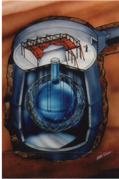
Figure 4.1: Example of a non-accelerator-based experiment. Heavy water targets can be protected from radiation background by installing them in deep-underground facilities. The target is surrounded by photomultipliers.
