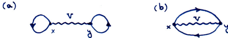
Figure 7: Two diagrams contributing to the perturbative interaction energy: (a) Hartree contribution; (b) exchange contribution.
