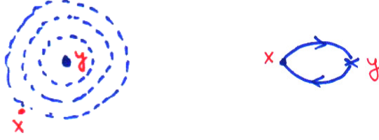
Figure 9: Left: A sketch of the experimental observation in the paper of Kanisawa et al. Friedel oscillations of the local density of states are observed around impurities. x is the observation point, y is the position of the impurity. Right: the diagram representing the first-order correction to the density of states due to the impurity potential.
