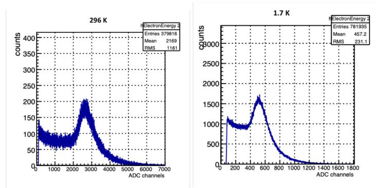
We achieved **sub-kelvin operation of commercial off-the-shelf scintillators** (Eljen EJ-204) and **silicon photomultipliers** (Hamamatsu S13370 VUV4), including single photon detection: DOI:10.1088/1748-0221/17/06/P06024.
