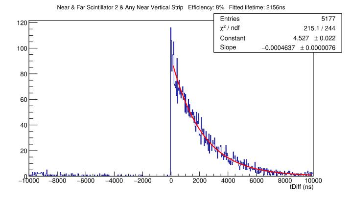
To improve the spatial resolution we are currently evaluating the operation of commercial 1 mm silicon strip detectors at **temperatures**  $T \approx 100$  mK. Our initial setup suffered from a low signal-to-noise ratio (SNR), limiting the detection efficiency to < 10 %. We **successfully detected** M eV **Michel**  $e^+$  as evidenced by the characteristic exponential decay spectrum of the time difference to the  $\mu^+$  entering the target chamber, notwithstanding.
