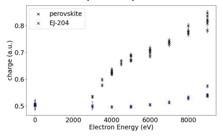
Tests with an electron gun show that **novel perovskite** (CsPbBr<sub>3</sub>) scintillators might provide a **significant improvement** over the aforementioned commercial EJ-204 scintillator at a **temperature of**  $T=4~\mathrm{K}$ .
