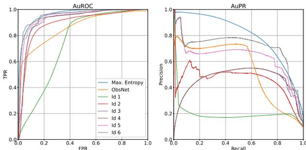
Figure 5: AuROC and AuPR curves of our ablated methods, ObsNet [10] and Max. Entropy [8] on RoadAnomaly [66]. Colors are consistent in the two plots and the Ids are the same as in Table 4.
