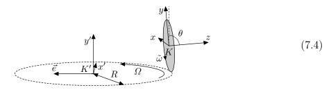
We define an accelerated frame K fixed to the centre of the coin with the z-axis aligned to its symmetry axis and the y-axis pointing in a largely upward direction. The inertial frame K' is fixed to the centre of the circle with the y'-axis aligned to the axis of the circle.
