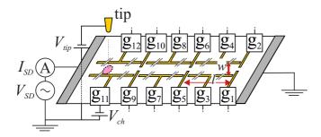
FIG. 1. Schematic of the gate geometry and measurement setup. Gates are labeled  $g_1$  to  $g_{12}$ . The pink area indicates the movable tip-depleted region.
