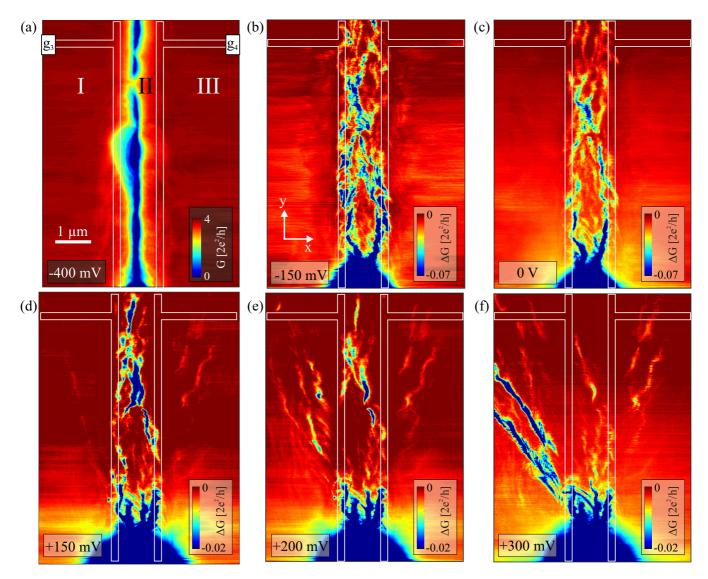
FIG. 3. Scanning gate images for different channel gate voltages as indicated in the images. (a) Conductance as a function of tip position for the QPC transmitting four spin-degenerate modes and  $V_{ch} = -400 \text{ mV}$  to electrostatically define the channel. (b)–(f) Series of scans with different, nondepleting  $V_{ch}$  showing  $\Delta G = G - 4e^2/h$  in color. The QPC transmits two spin-degenerate modes in the absence of the tip.
