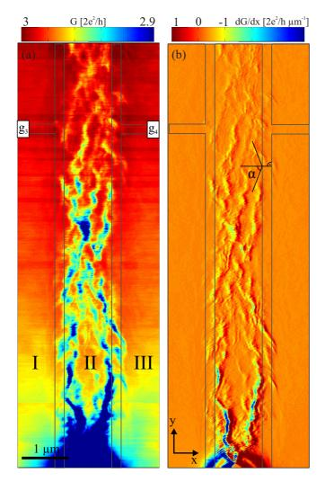
FIG. 2. (a) Conductance G(x, y) of QPC 1 on sample A. Gray solid lines mark the outlines of the gates. Roman numbers label the channel region (II) and the two regions outside the channel (I and III). (b) Derivative dG(x, y)/dx of the data in (a).
