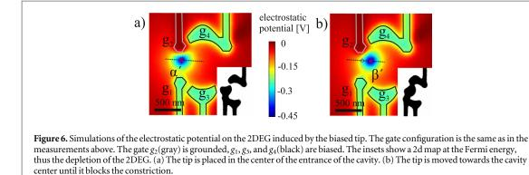
was modeled as a dielectric with  $\epsilon = 13$ . The tip, implemented as a metallic cone with a hemisphere with radius 50 nm at its end, is placed 70 nm above the surface. We determine the induced density in the 2DEG and consider regions to be depleted if the induced density exceeds the sheet density of the electron gas.
