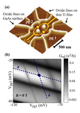
FIG. 1 (color online). (a) SFM micrograph of the structure (details in the main text). (b)  $G_{\rm sd}$  as a function of  $V_{\rm pg1}$  and  $V_{\rm pg2}$  representing the charge stability diagram of the two QDs. The finite-bias measurements in Fig. 2 were taken along the dashed lines.
