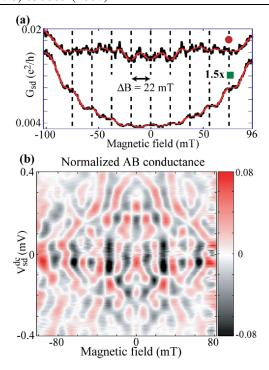
FIG. 3 (color online). (a) B dependence of the differential conductance for gate voltages set to the center of the hexagon in Fig. 1(b). Bottom trace: low dc bias voltage (square, c.f. Fig. 2); top trace: high dc bias voltage (dot). (b) Normalized AB conductance  $g_{AB}(B, V_{bias})$ .
