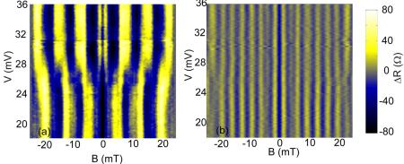
FIG. 3 (color online). (a) Evolution of the AB oscillations upon changing the plunger gate voltages  $V_{pg1} =$ -120 mV - V;  $V_{pg2} = -120 \text{ mV} + V$ . (b) Filtered h/2e oscillations as a function of the plunger gate voltages, showing the local minimum at B = 0 T at all gate voltages.
