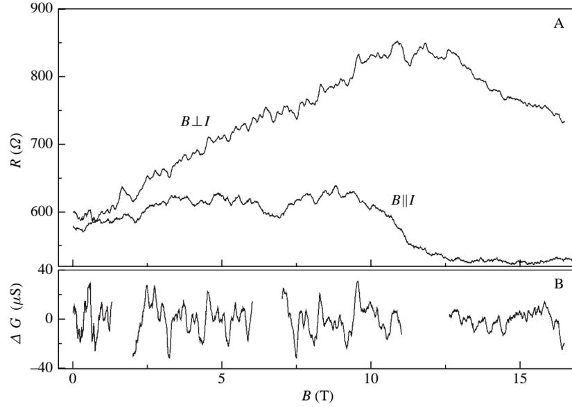
**Fig. 2.** A Two magnetoresistance curves from wire B. In both,  $B$  is applied parallel to the 2DEGs, but the orientation of  $B$  relative to  $I$  is changed. B The bare UCF in wire B for  $B \perp I$  in the different magnetic field ranges of interest, as obtained by subtracting a smooth background from the original  $R(B)$ .
