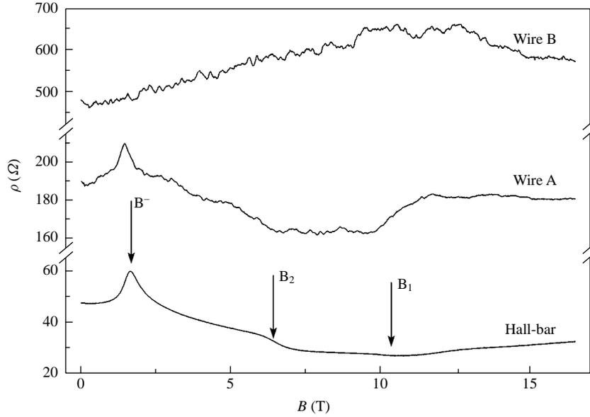
**Fig. 1.** Magnetoresistance in a magnetic field,  $B$ , applied in the plane of the QW and normal to the current for a macroscopic Hall-bar sample and wires A and B.
