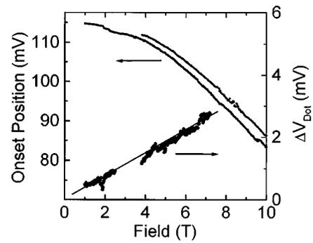
FIG. 3. Voltage positions and the splitting ( $\Delta V_{\text{dot}}$ ) of the onsets of the spin split peaks vs magnetic field. No values are plotted between 2.5 and 4 T, as the splitting is not clearly defined.
