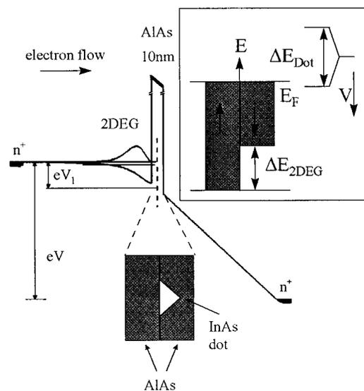
FIG. 1. Conduction band potential profile of the device under bias. The lower inset shows the orientation of a single dot in forward bias, and the upper inset a schematic diagram of the spin splitting in the dot and partial spin polarization of the 2DEG in a magnetic field. The effect of applying a voltage across the device is to move the dot energy levels down relative to the Fermi level of the 2DEG.
